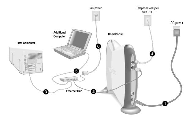
**Note:** The HomePortal has an auto-crossover port. You do not need to use a special crossover cable or make any changes to the configuration of your HomePortal, Ethernet hub, or switch. The HomePortal will establish the type of port needed during setup.
